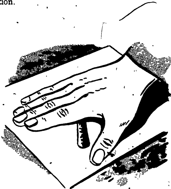
Figure 1-14. Rolling the soil, plastic limit test.
